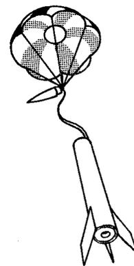
each of your parachutes. Pre-test the size of the parachute for safe recovery by hand-tossing the model into the air with the parachute hand-wadded but outside the body tube or by dropping the rocket with the parachute unfurled from a high elevation, such as a second or third floor window.
