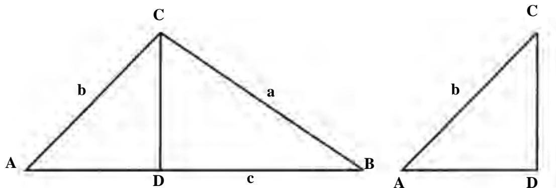
The altitude of the rocket is the distance from D to C in the diagram. The angle formed by the meeting of AB and CD is a right angle. The sine of an angle in a right triangle is the relation of the opposite side to the hypotenuse. The value of the opposite, CD, needs to be determined.
