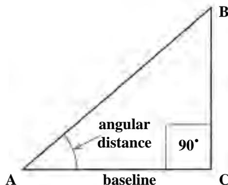
The tangent is used to determine altitude because the tangent of an angle in a right triangle is the ratio of the opposite side to the adjacent side. In this example, the adjacent side is the distance along the baseline. The opposite side is the distance from the launcher to the rocket's maximum altitude. Tangents can be found in the Table of Tangents in the Appendix.
