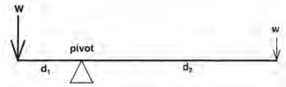
Not only does the magnitude of the force affect the balance, but also how far away from the pivot point the force acts. The smaller force “w” acting at a distance  $d_2$  has the same effect of a larger force “W” acting at a distance  $d_1$ . This is just like the aerodynamic forces acting on a rocket. Forces acting at a distance away from the pivot point (or CG for a rocket) create a “Moment”; force times distance. In the example above, the moments created by W and w are balanced.
