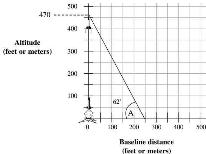
If we assume that the rocket flight is vertical, we can call angle C (in the previous figure) a right angle,  $90^\circ$ . B is equal to  $90^\circ$  minus A because the sum of the angles in a triangle is  $180^\circ$ . By definition:
