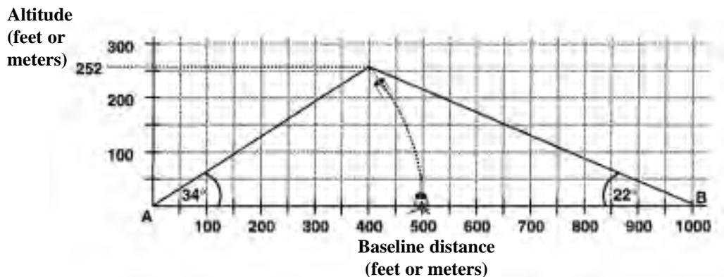
Plot elevation angles A and B, then extend them until they intersect. The point of intersection extended to the vertical axis is the rocket's altitude.
