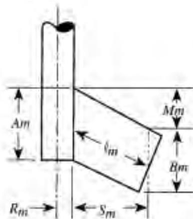
\*NOTE: Dashed line refers to fin tip being parallel to fin root and idealizing actual fin area.
