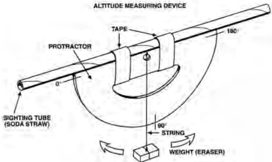
You will be constructing a device that looks like the one in the diagram. Tape the straw across the top of the protractor as shown. The straw will act as a sighting tube. Secure the string to the protractor by slipping it under the straw and around. Tie it to itself and tape it to the back of the protractor. Tie the eraser at the opposite end of the string so that it can act as a weight.
