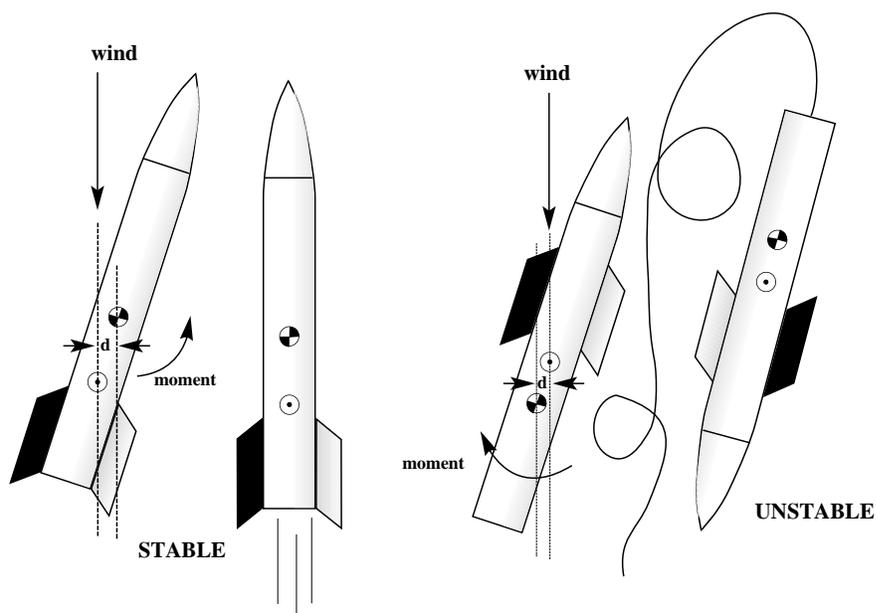
fins. This will counteract the rotating forces and the model will continue to fly straight. If the center of pressure is ahead of the center of gravity, the air currents will exert a greater force against the nose end of the rocket. This will cause it to rotate even farther. Once it has begun rotating it will become unstable.
