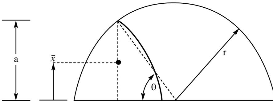
$\bar{x} \approx 0.38a$  (for a typical nose cone)
