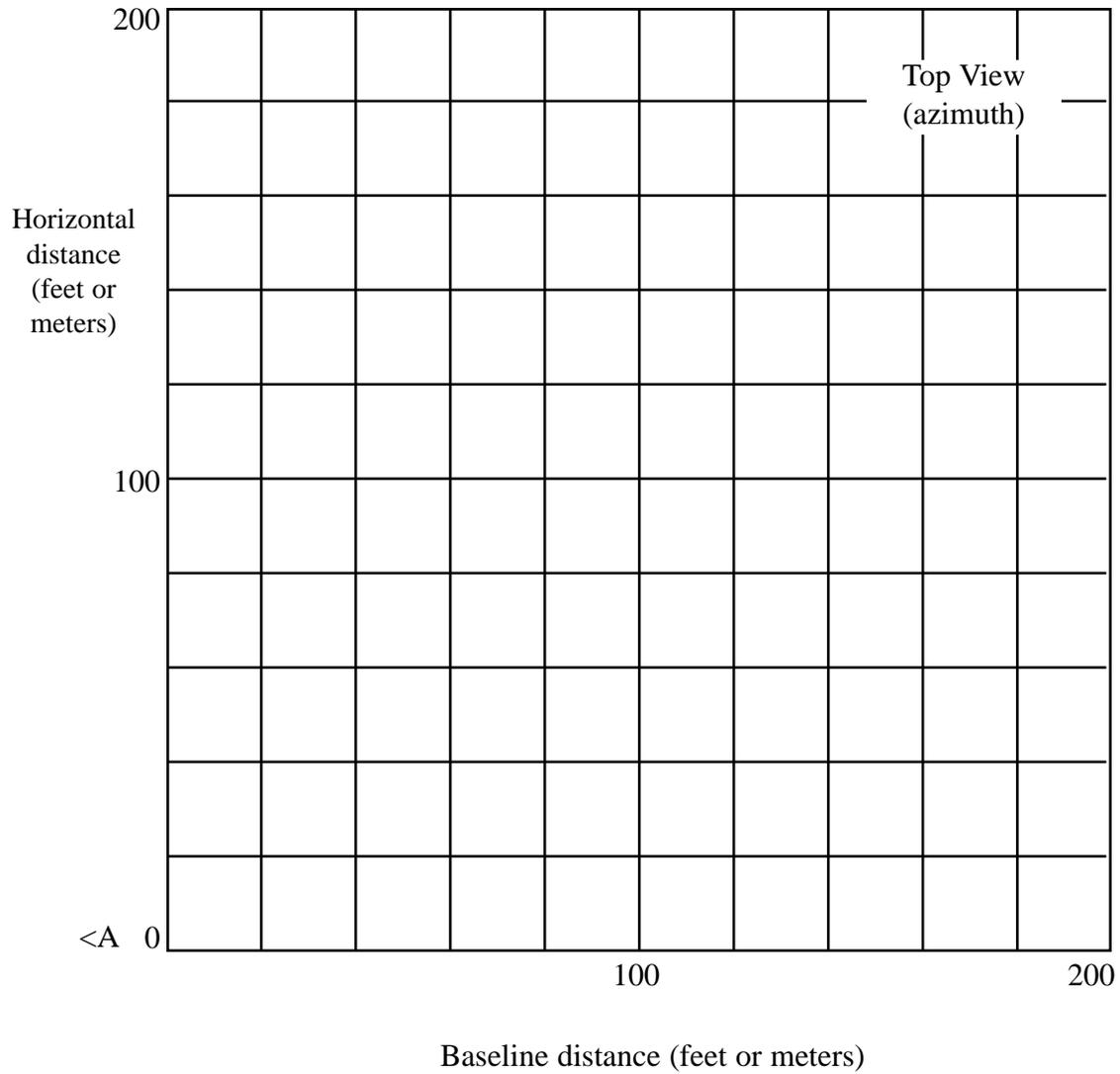
Plot the baseline distance and azimuth angles for the top view graph to find the unknown horizontal distances (a and c).
