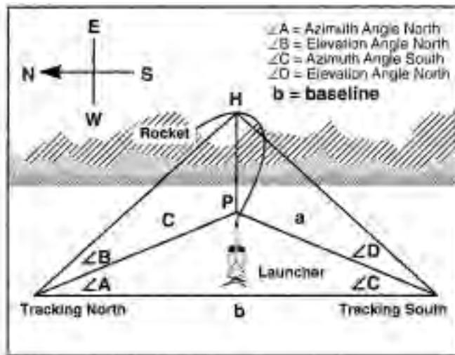
For this system a two station tracking type scope is needed. The two trackers are set up on a base line with the launch pad roughly halfway between them, but off the baseline to one side. Both scopes are then “zeroed” on each other. This means that when looking through the scope toward the other, the azimuth and elevation angles should both read zero degrees. The rocket is then fired and both trackers sight the model until it reaches apogee, at which point they stop and record the angles.
