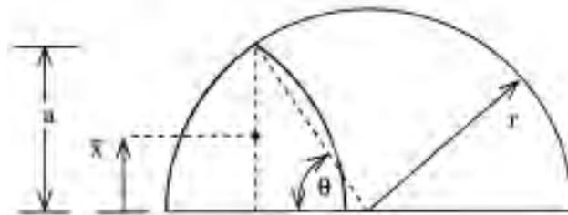
Calculating the center of pressure of rocket outline
