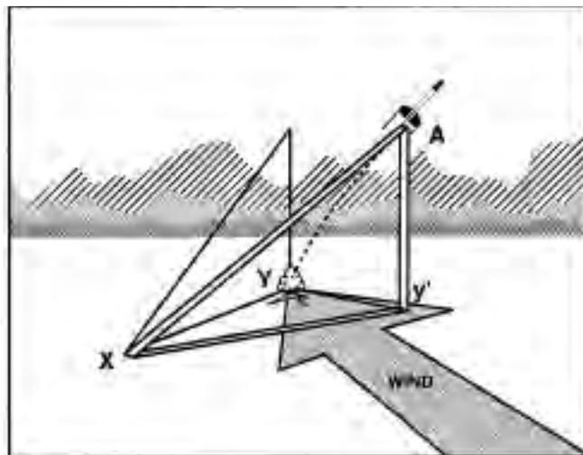
By observing the proper relation between wind direction and the position of the tracker, we can generally determine with 90% or better accuracy the altitude the rocket reaches from data given by only one elevation tracker. Thus, on a calm day with a good model, almost perfect accuracy can be approached.
