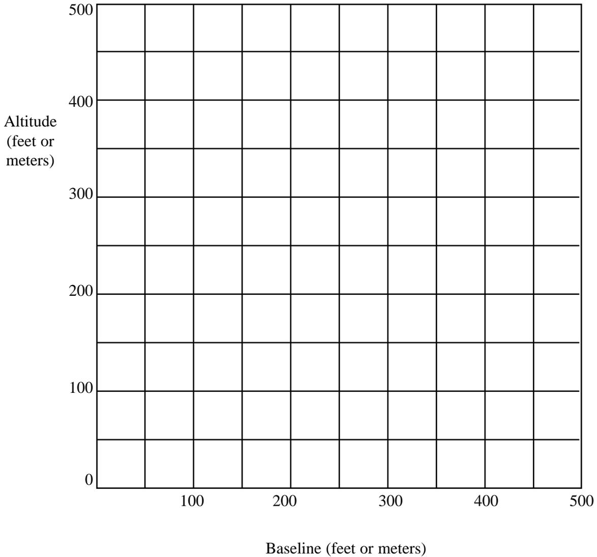
Use the horizontal axis to plot the baseline distance (distance from launcher to tracker).
