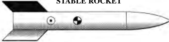
Younger students can be helped to understand the center of pressure by finding the balance point of a number of geographic shapes used in the construction of model rockets. (See Appendix ) This balancing point, referred to as the centroid, describes the geometric center of area for a given shape. The term  $\bar{x}$  locates the centroid from a reference point.
