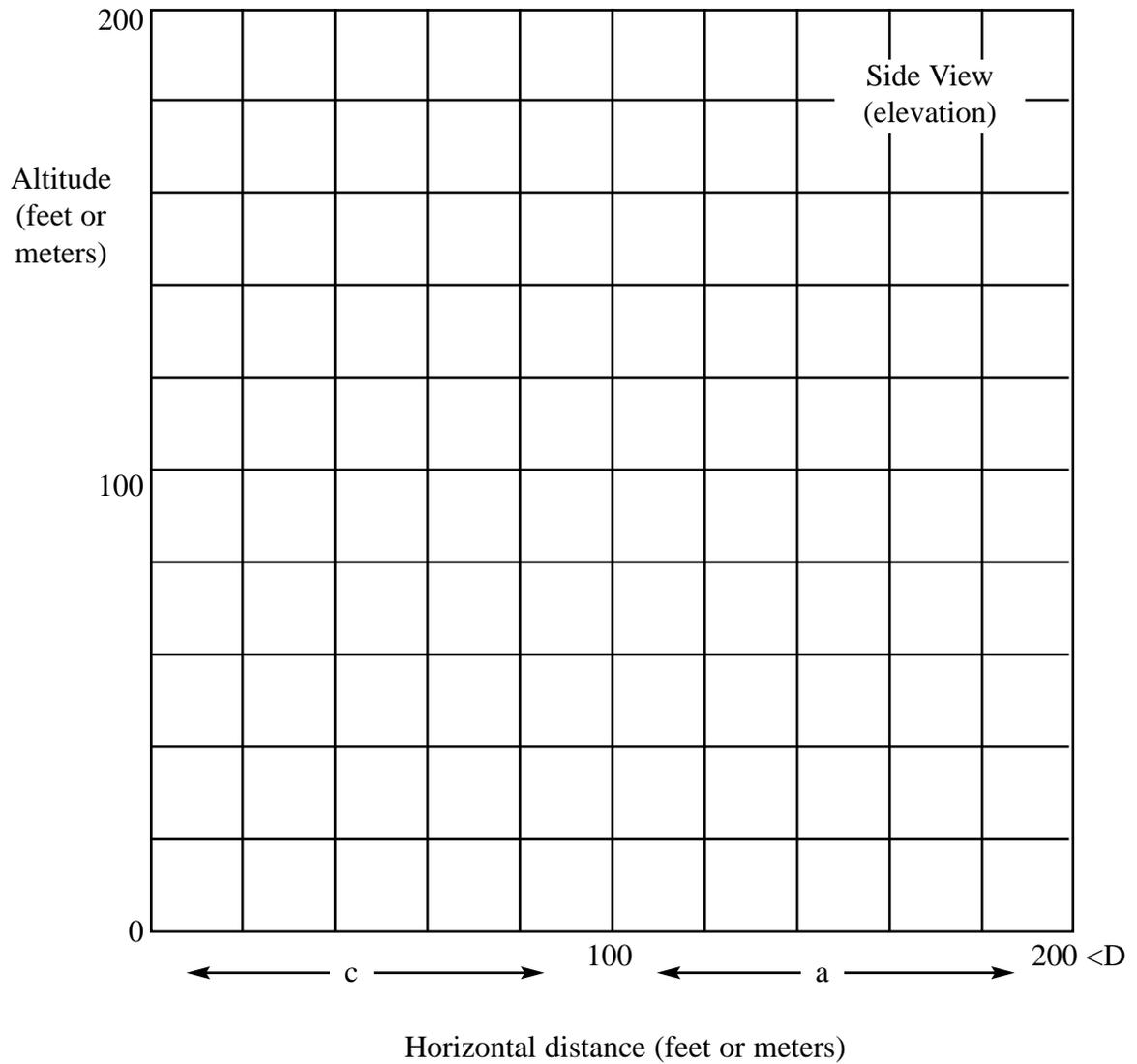
Plot the elevation angles and distances  $a$  and  $c$  to graphically depict height  $PH$ . When the elevation angles are plotted there will be two different values of  $PH$  so they must be averaged.
