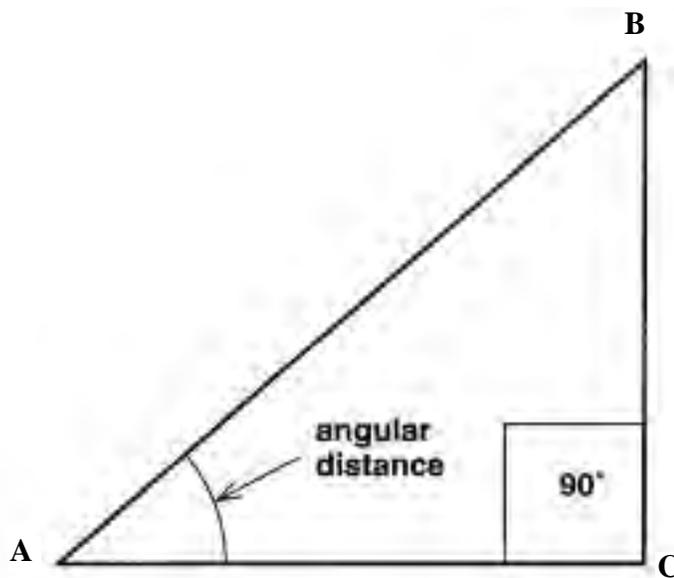
Describe the location of the launch pad, C, the tracking station, A, and the rocket at apogee, B. AC is the baseline. Angle A is the angular distance.
