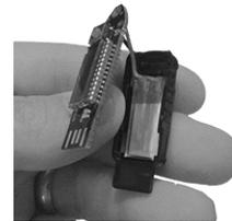
Lay the battery in the bottom case, with the colored, complicated part of the battery down and the wires away from the USB tray.
