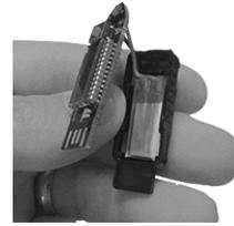
The battery includes embedded safety circuitry, but you should be aware that Lithium Polymer batteries are capable of generating significant current. Take extra care to not allow shorts to occur during repair.
